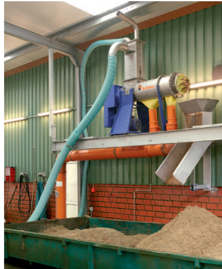
OptiPress II for substrates with higher dry matter content and a coarser structure
